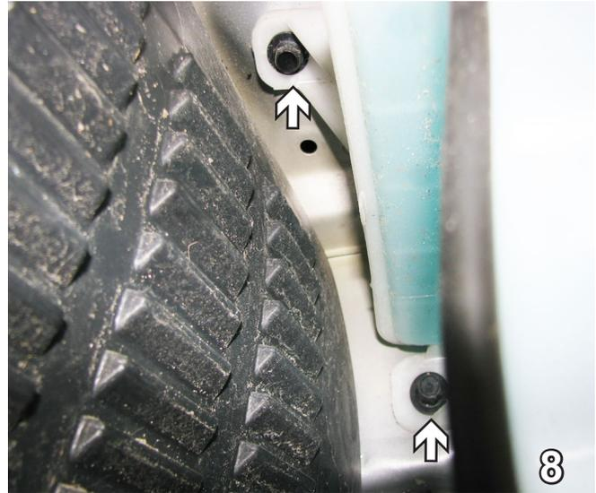
8. Using a 10MM socket on the left side of the washer reservoir remove two bolts. Set bolts and reservoir aside to be reinstalled later.
