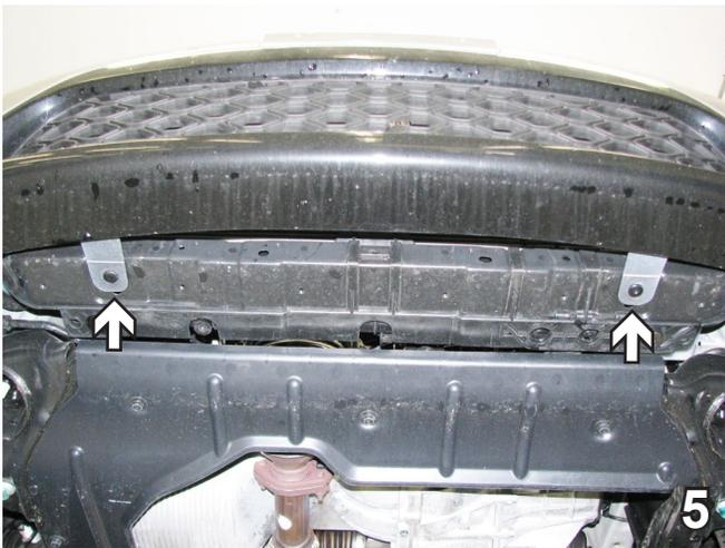
5. Underneath the fascia in the center remove the two plastic push pins. Set fascia and push pins aside carefully to be reinstalled later.
