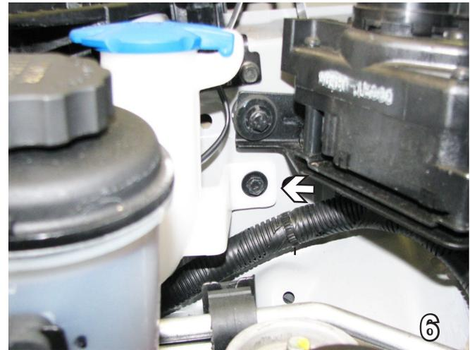
6. On the passenger side, using a 10MM socket remove one bolt from the top of the washer reservoir. Set bolt aside to be reinstalled later.
