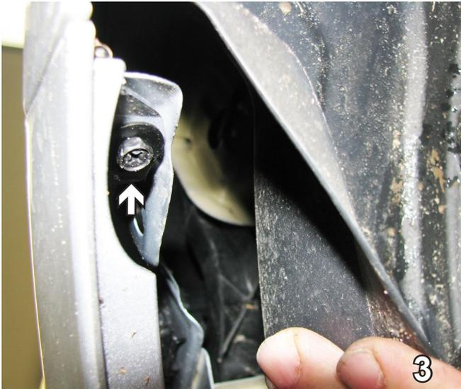
4. Pull the plastic wheel well cover back, using an 8MM socket remove the bolt underneath. Do this to both sides of the vehicle. Set the bolts aside to be reinstalled later.
