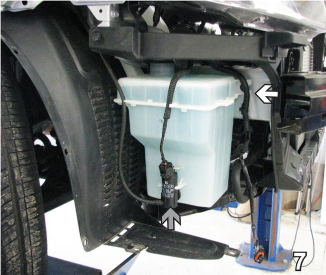
7. Using a 10MM socket, remove one bolt from the right side (white arrow) of the washer reservoir. Set the bolt aside to be reinstalled later. Unplug the electrical connection and the hose and cap the hose (gray arrow).
