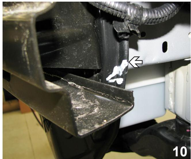
10. Go up 1/2" from where the cut started flush with the bottom of the frame. Cut out a v notch to the point of intersection with the side of the frame. Do this to both sides of the vehicle.
